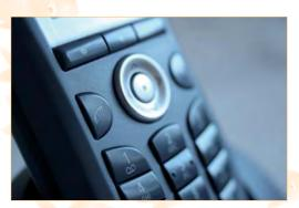
Telephones for voice over WiFi are also an alternative to DECT. The innovaphone IP62 is the first VoWiFi handset, operating on all IEEE-802.11a/b/g/n networks. The innovaphone IP62 fully supports the IEEE-802.11n standard thus supporting the deployment of voice over the network without degrading the performance of the network. The SIP and H.323 protocols are fully supported; therefore,
