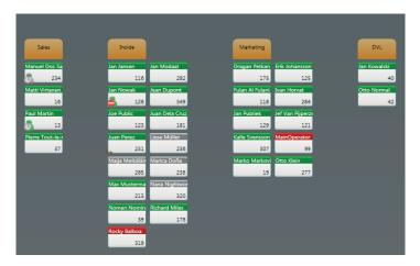
A server is not needed to run the innovaphone Operator. The Operator connects directly with the innovaphone PBX over SOAP.
