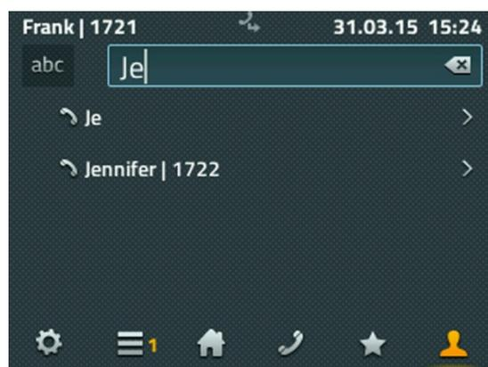
When using the IP111, IP112 and IP222 phones, a shift key is at the top left to enter numbers and switch between capital/small letters. The backspace key on the right of the input box deletes the last character before the cursor.
