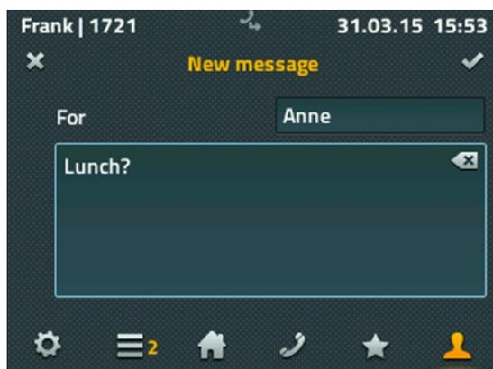
A full keyboard is also available for writing messages. Press the tick icon at the top right to send the message. A message appears briefly for about 2 seconds showing the send status - if successfully sent: a simple "OK" appears, if unsuccessful: "Operation failed". Most "operation failed" cases are due to the remote terminal not being capable of receiving messages.
