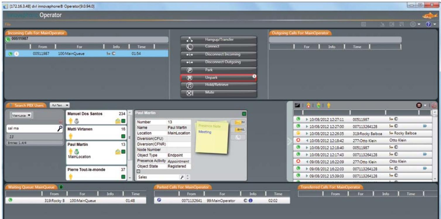
The innovaphone Operator is a modern computer-based telephone switchboard for the innovaphone PBX. It can access the innovaphone PBX's waiting queues and it can forward calls. These calls can be switched both with or without consultation across multiple sites (blind transfer).
